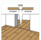
2. Install the laminate **according to the installation instructions**, with an expansion gap of 8-10mm. Do not install laminate under (fixed) heavy objects such as a bathtub, integrated cabinets,... Install heavy or fixed furniture before you install the floor.
