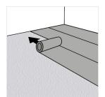
Underlay: The installation starts with a BerryAlloc underlay with integrated moisture barrier. Use the BerryAlloc Excellence Impact+ or the Excellence Plus underlay for the best result. Read the BerryAlloc Underlay guide for more info.
